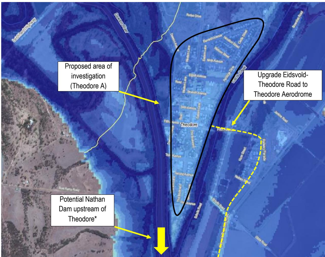
**Image: Proposed area of investigation, potential road upgrade and potential upstream mitigation option with 1% + CC AEP flood inundation depths shown**
