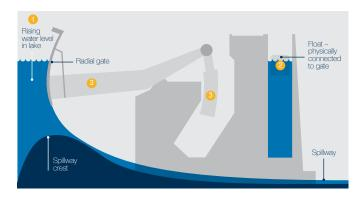
The gates have a series of chambers and counter weights that are influenced by the water level in the storage. When the water level rises above 216.259m AHD the gates will begin to open.
