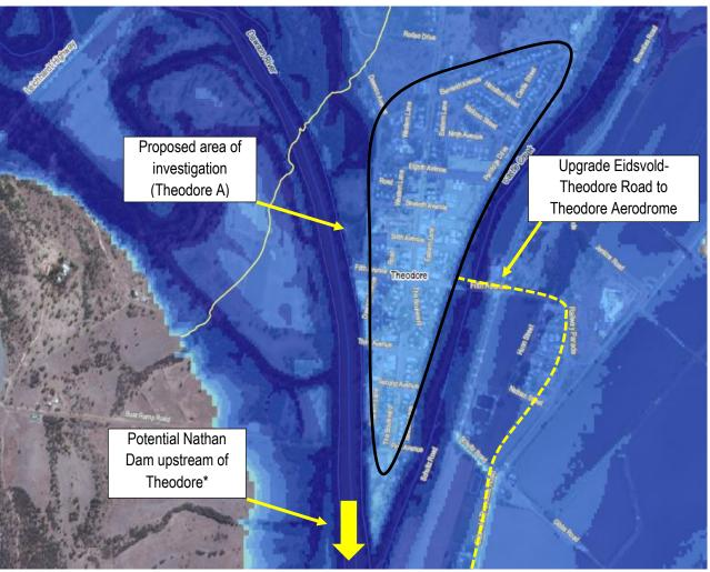
Image: Proposed area of investigation, potential road upgrade and potential upstream mitigation option with 1% + CC AEP flood inundation depths shown
