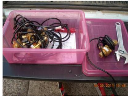
CO<sub>2</sub> gas cylinder regulator, regulator hose and spanner
