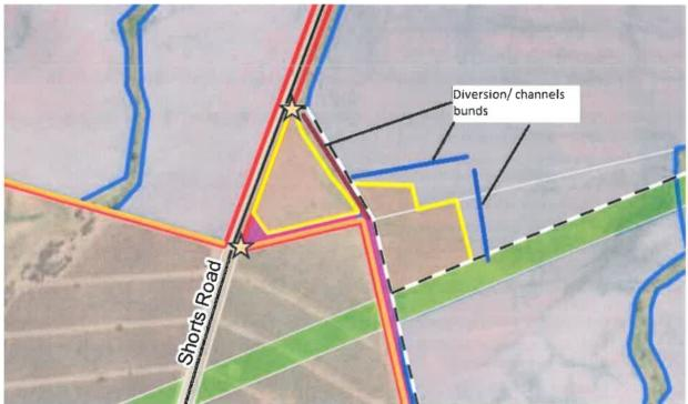
Figure 5: Proposed diversion bunds/ channels for the laydown area and associated infrastructure
